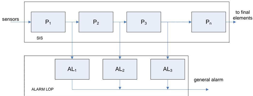
**Figure 3. Safety Instrumented System monitored by alarm annunciator.**
