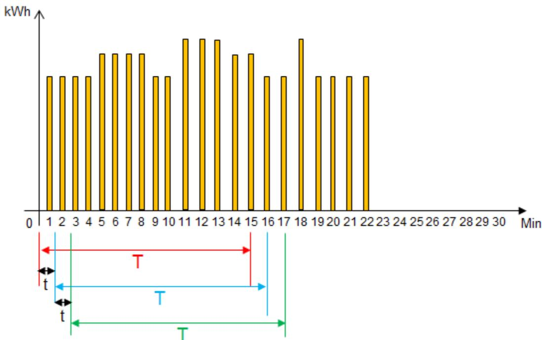
1. As shown in the above figure, when  $t=1$ , the frequency to record energy consumption will be once per minute. When  $T=15$ , each 15 minutes the sum of the energy consumption measured every minute ( $t=1$ ) will be calculated.
