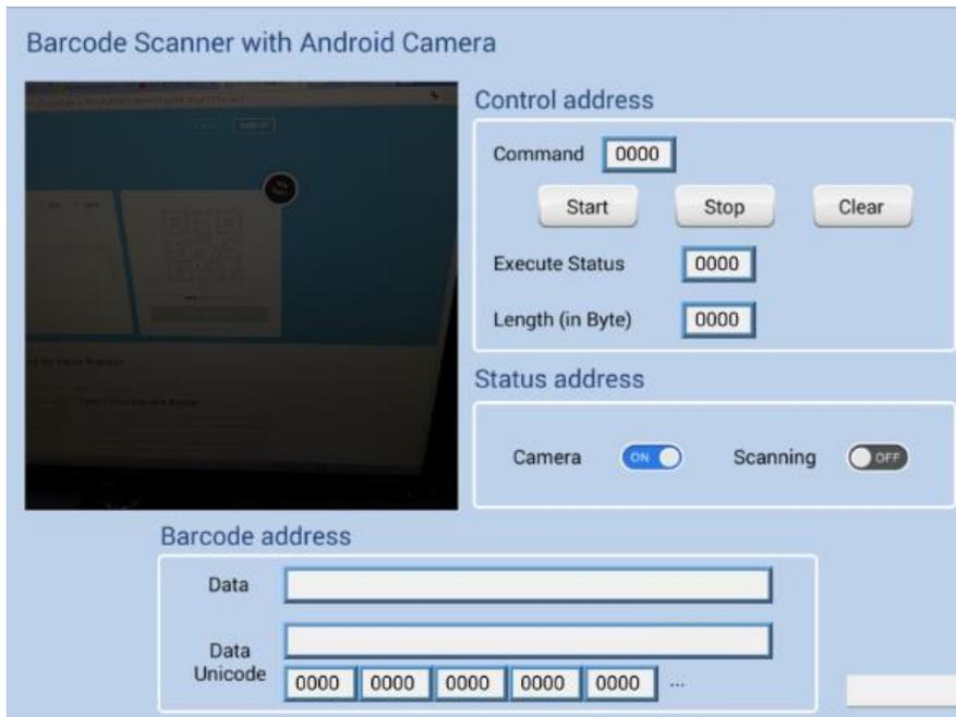
2. Tap Start button, the status of Scanning turns ON, the display turns bright, and is ready for scanning.
