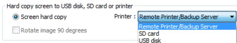
7. Place the Function Key object in the common window (window no. 4) so that screen hardcopies can be captured anytime when needed.
