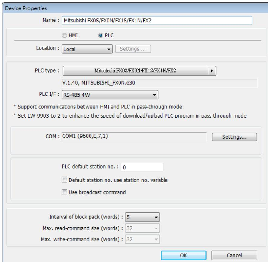
5. A new device is added to the [Device List].
