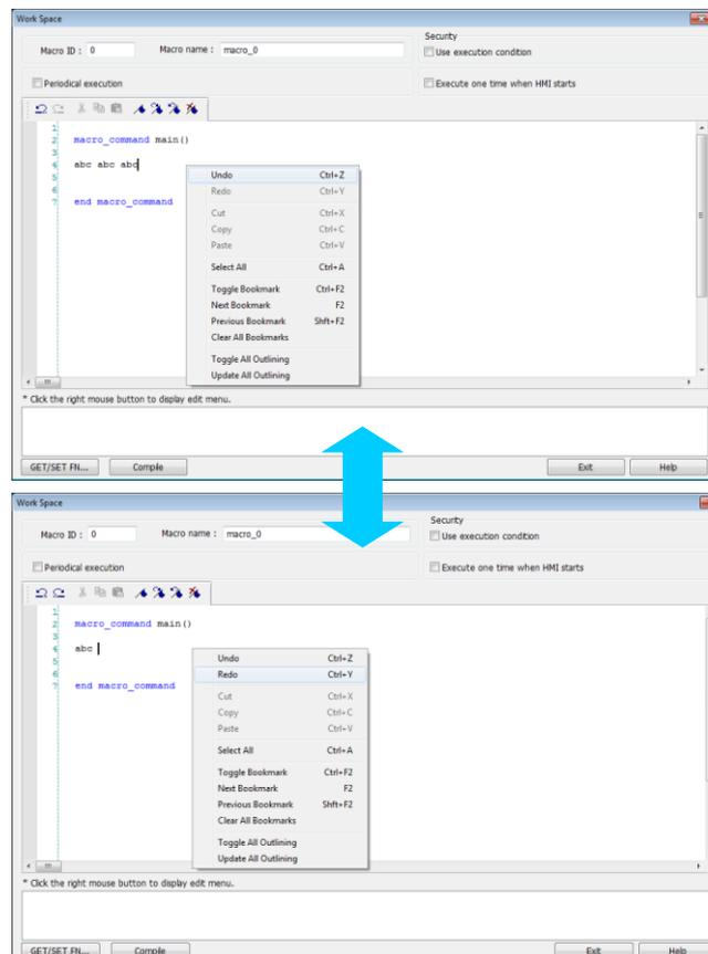
5. Select a word in the editor to enable the [Cut] and [Copy] function. After [Cut] or [Copy] is performed, [Paste] function is enabled.
