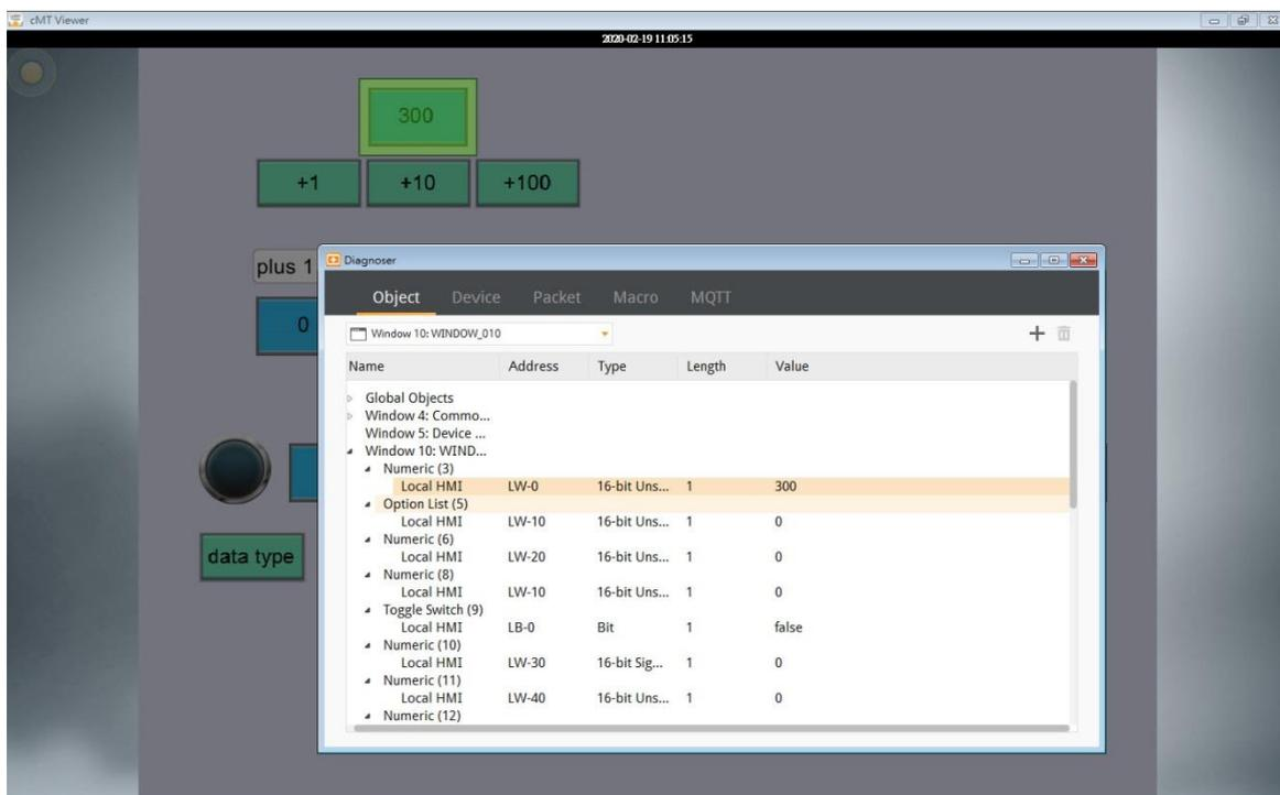
4. The value of an object can be changed by double-clicking on it in cMT Diagnoser window.
