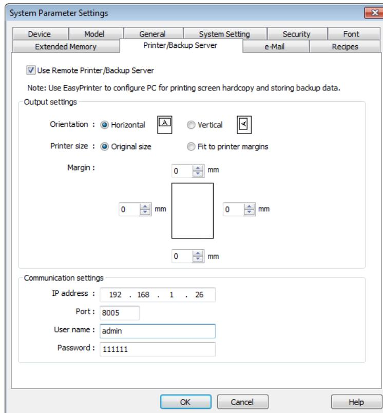
3. Under [Output settings] set appropriate values for left / top / right / bottom margins. (The margins are all set to 15mm in the example.)
