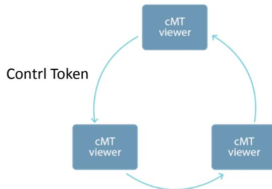
One cMT / cMT X HMI can be simultaneously controlled by multiple cMT Viewer clients. To ensure system safety by preventing an object to be controlled by multiple clients simultaneously, a control token can be set. Only one cMT Viewer client can acquire the control token at a time, and only the cMT Viewer client that acquires control token can operate the object. The rest of the clients can acquire the token one by one when the token is not occupied.
