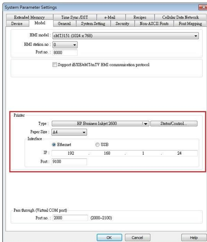
2. Select a printer type. To add a new printer, place the printer's PPD file in the ppd folder under EasyBuilder Pro installation directory, and then click [Refresh].
