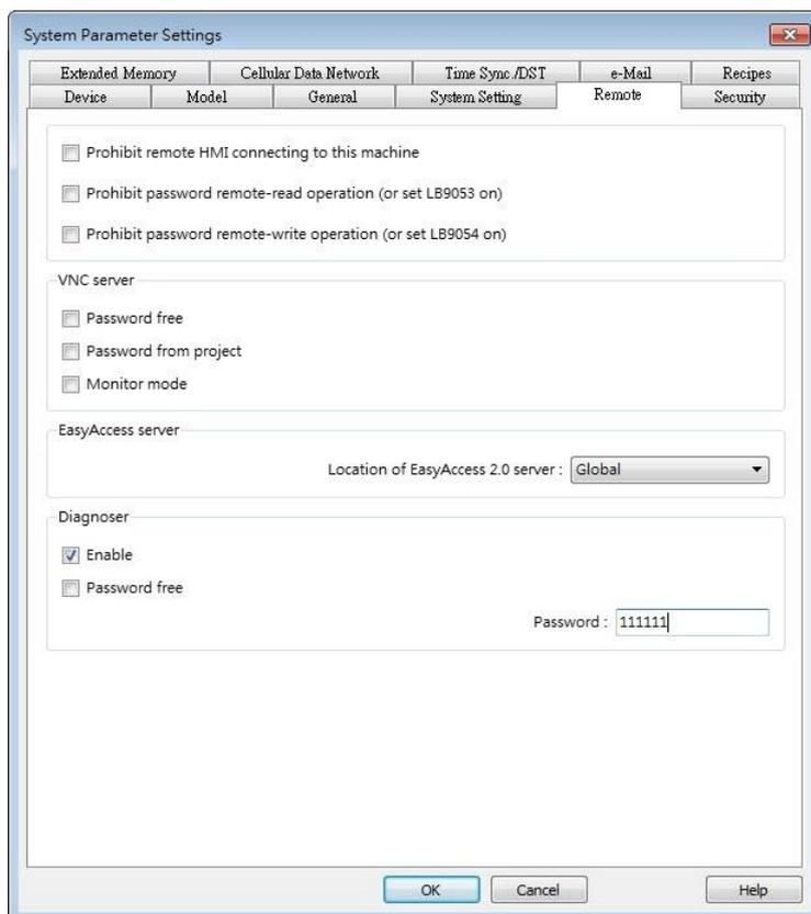
After downloading the project to HMI, cMT Viewer can open cMT Diagnoser. If [Password free] is not selected in Remote tab in previous step, a password is required for running cMT Diagnoser.
