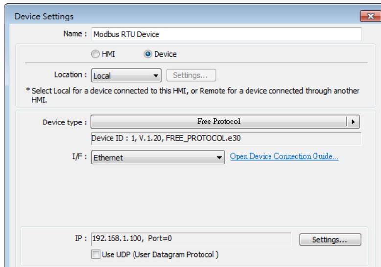
Suppose that the HMI will read the data of 4x\_1 and 4x\_2 on the device. First, utilize OUTPORT to send out a read request to the device. The format of OUTPORT is:
