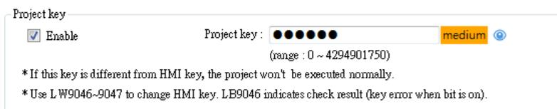
Enable and set the [Project key] (password range: 0 ~ 4294901750). System registers LW-9046 ~ LW-9047 (32-bit) can be used to set the [HMI key] for HMI. The values in LW-9046 and
