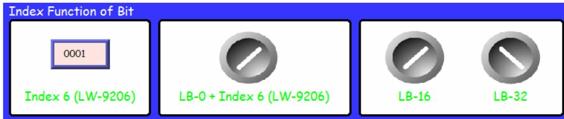
If Index 6 (LW-9206) is set to 1, then switch [LB-0 + Index6] reads LB-16 which is in ON state.
