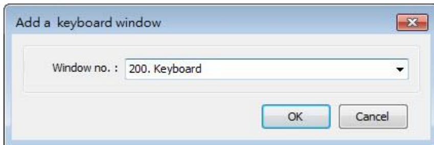
5. After the keyboard window is added, when you create Numerical Input and ASCII Input objects, “200. Keyboard” can be found in [Data Entry] » [Keyboard] » [Window no.]. The [Popup position] is for designating the display position of the keyboard on the HMI screen. The system divides the screen into 9 areas.
