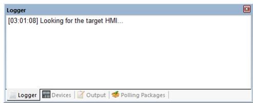
6. The possible reason of not being able to get connection with HMI can be failure in executing simulation on PC. Another reason is that the Port No. used in project for simulation on PC is incorrect (or occupied by system). Please change Port No. as shown, compile project then do simulation again.
