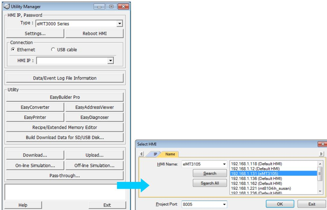
10. Download the project to HMI and start the project. If EasyDiagnoser is unable to get connection with the HMI to be watched, it is possible that HMI power is not ON, or Port No. is incorrect. This may cause EasyDiagnoser to connect then disconnect with HMI continuously. Please check the Port No. in EasyDiagnoser settings.
