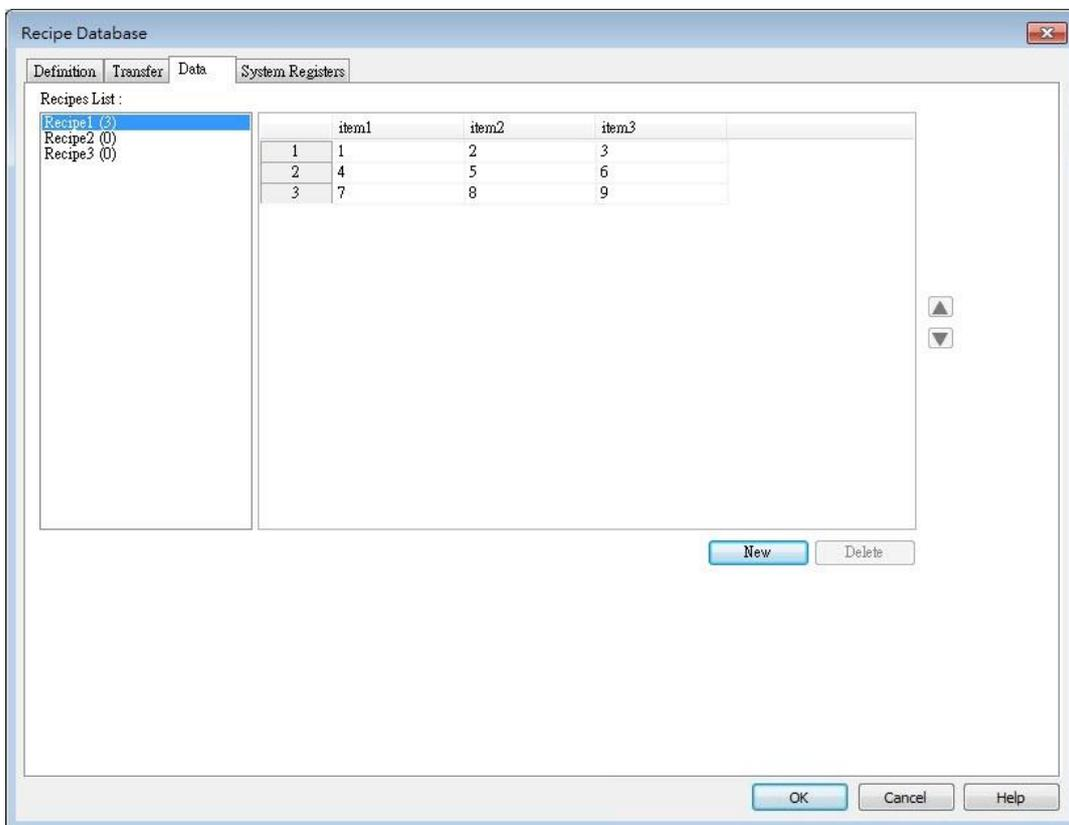
In the example shown above, Recipe created in the Definition tab can be found. Items shown on the right hand side come from item names added in Definition tab. Data of each item name can be configured in this tab following the data type defined in the Definition tab.
