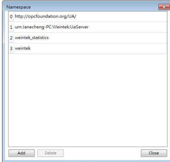
Object types of a device can be added to or deleted from this list.
