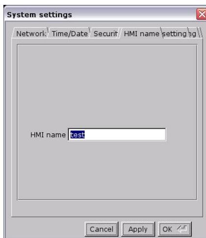
2. On PC, select the HMI name and start downloading. To use [Search], enter the HMI name first to search for the HMI. [Search all] searches for all HMIs in the same subnet network.
