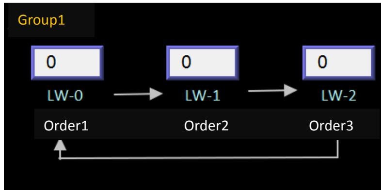
2. When finish entering data in the last object, to end data entry of all objects, please select [Stop sequential input function after input] check box.
