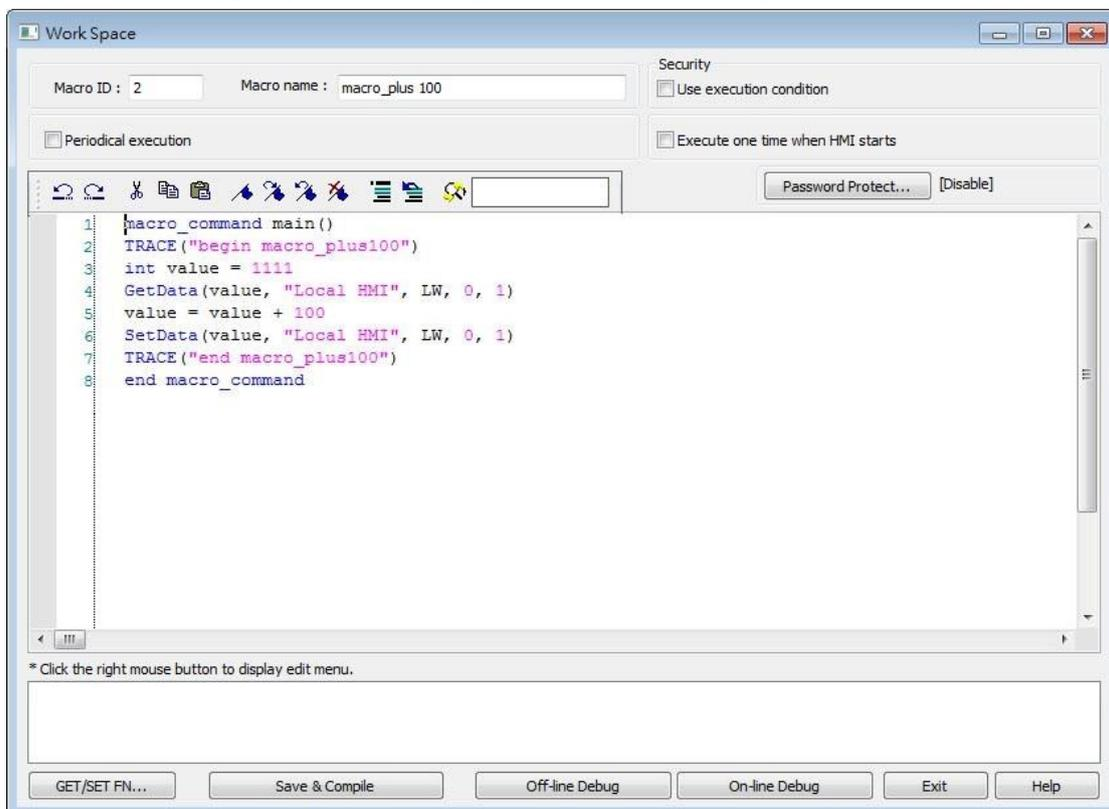
Click [On-line Debug] or [Off-line Debug]. Software will generate a Macro Debug File. Also,
