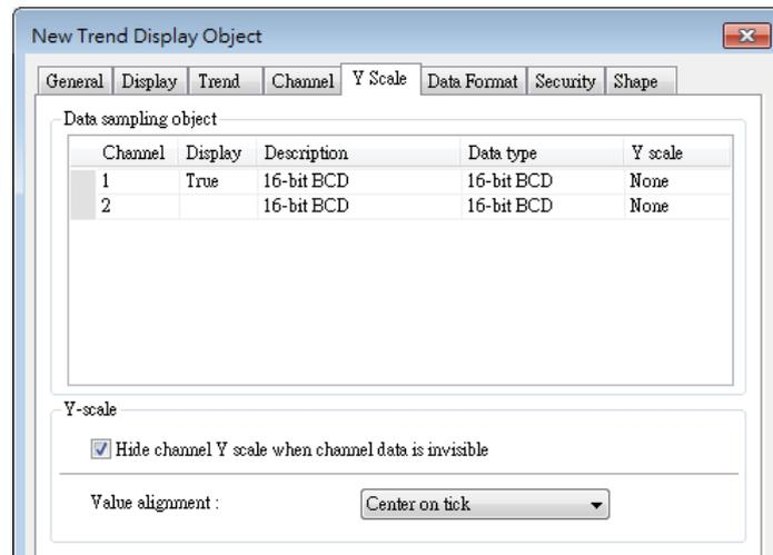
The scale along the Y axis of a specific channel can be displayed. To enable Y Scale, [Grid] should first be enabled in [Trend] tab.
