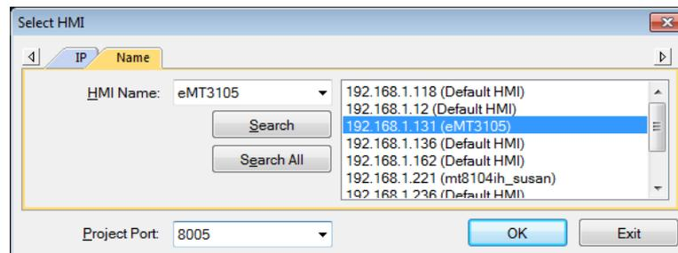
The three consecutive ports of the project port no. are preserved for HMI communication. In the setting above as an example, Port No. is set as 8005. Port 8005, 8006 and 8007 should be reserved. In this case when executing simulation on PC, please make sure that these ports are not occupied by other programs.
