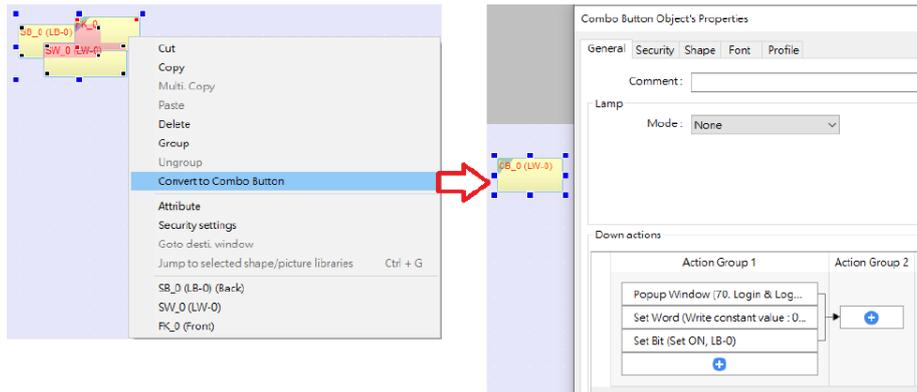
After [Convert to Combo Button] is clicked, a review window shows for users to review the actions that can be triggered by the Combo Button. Actions that are not highlighted can be merged; actions that are highlighted in yellow will be automatically adjusted to meet merging condition; and actions that are highlighted in red cannot be merged. The user can move the mouse cursor to the yellow or red area to see explanations.
