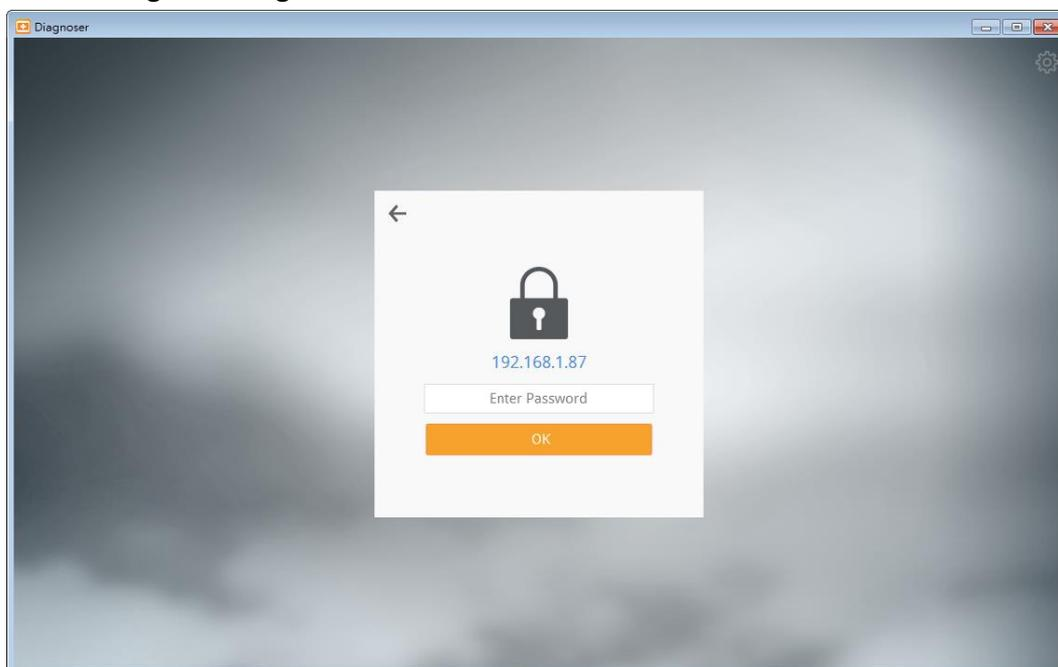
3. Execute cMTDiagnoser.exe, which can be run independently, in EasyBuilder Pro installation directory, and find an HMI to connect to.
