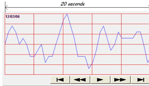
Select [Time] for [X axis time range] and go to [Trend] » [Grid] and enable [Time scale]. Please refer to [Time scale] in the later section.
