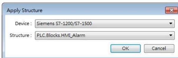
Structured node set under a device can be added, only if the device is a symbolic PLC and has structured data type defined.
