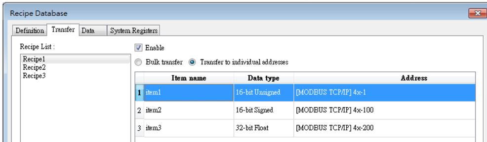
Under this mode, the data type setting of each destination addresses must also follow those of the corresponding recipe item. In the settings shown above, the data type of address 4x-1 should be 16-bit Signed, and 4x-100 should be 32-bit Signed, and so on.
