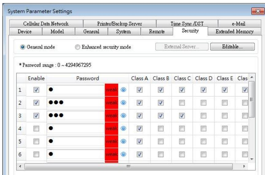
Up to 12 sets of user and password are available. Password should be one non-negative integer. Once the password is entered, the objects that the user can operate are classified.
