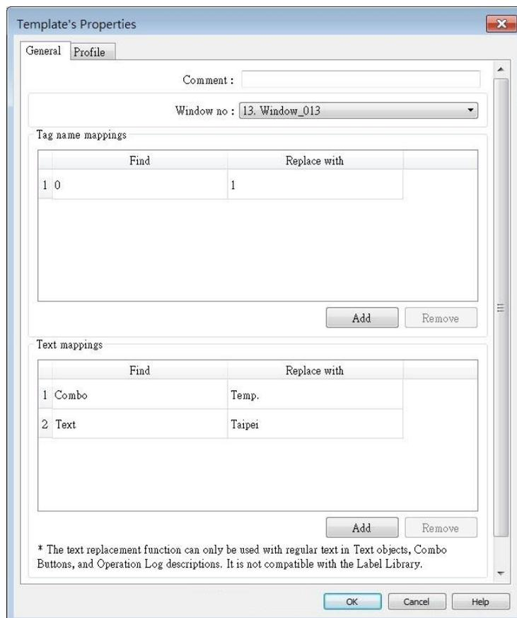
8. After compiling the project, EasyBuilder Pro will replace any tag names containing “0” with “1” for objects in the Template Window that use them. This means that “Tab\_0” will be replaced by “Tag\_1”. The text mapping feature will also replace object comments, text contents, and text labels according to the settings defined in the Template object.
