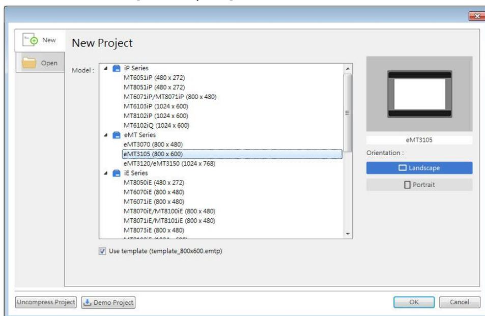
3. Click [New] button in the Device tab and select a device.
