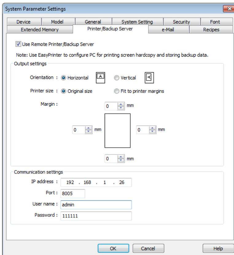
3. Under [Communication settings] fill in the [IP address] of the printer server according to the settings in EasyPrinter. Set the [Port] to “8005”, [User name] to “admin” and [Password] to “111111”. (Note: These are default values.)
