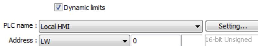
Set [Address] to LW-0 and create two Numeric objects for entering the low / high limit. The address that controls the low limit is LW-0; the address that controls the high limit is LW-1. Let's suppose the data is between 0 and 30; set the [Low limit] to 0 and the [High limit] to 30, the trend curve is displayed as shown in the following figure.
