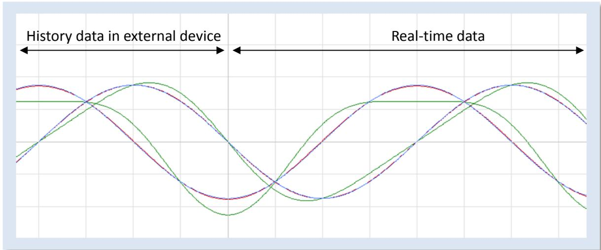
For other series, when displaying the sampled data in Trend Display object, it is necessary to select from Real-time mode or History mode and the two modes cannot simultaneously be displayed in one object.
