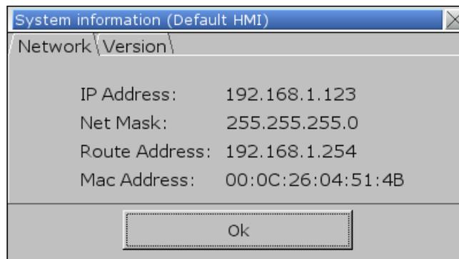
2. On PC, enter the HMI IP address: <ftp://192.168.1.123> (example), then log in by the user name: uploadhis, and enter the HMI [history upload password] (if not changed, the default password is 111111). Or, directly enter <ftp://uploadhis:111111@192.168.1.123/>
