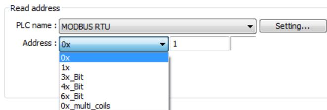
Since the server is an HMI, the corresponding read and write addresses are listed below :
