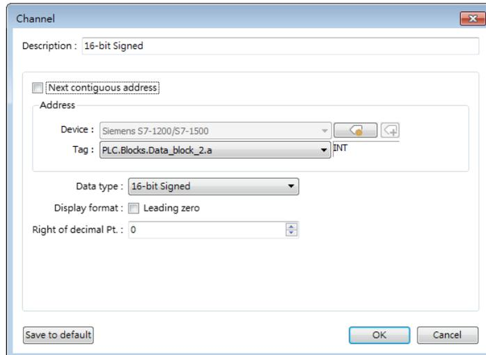
Please note that when contiguous address setting is used for a tag-based PLC driver, only one-dimensional arrays are supported.
