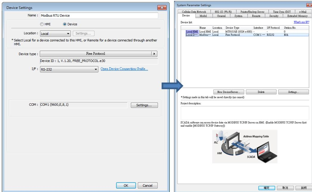
2. The interface of the device (I/F) uses [RS-232]. If a MODBUS TCP/IP device is connected, the interface should be [Ethernet] with correct IP and port number as follows:
