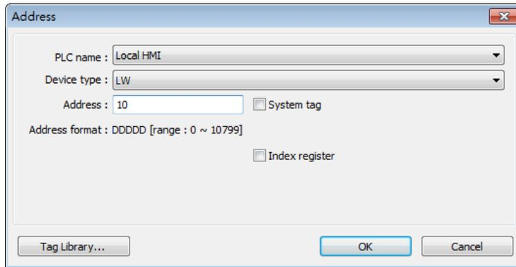
If select [**Index register**] check box and set [Index] to [INDEX 0 (16-bit)], the system will read / write [LW(10 + value in Index Register 0)].
