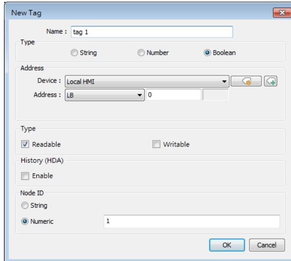
Add a new tag for the client to monitor or control. Two types of tags can be added: Data Variable and Property.
