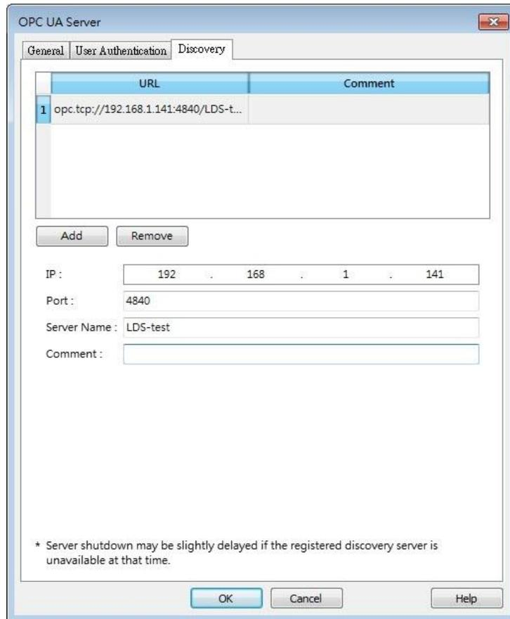
When configured, OPC UA server will register to the Local Discovery Server (LDS). OPC UA Discovery service is used to simplify server location maintenance when there are many OPC UA servers in the network. An OPC UA client can access one LDS Server and obtain all registered OPC UA server.
