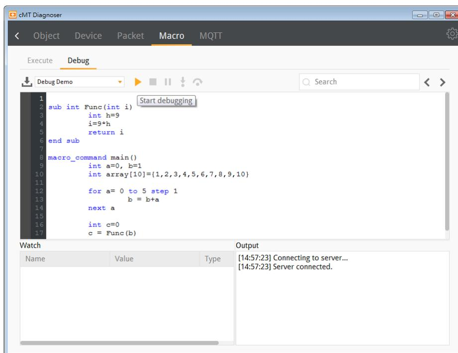
2. Set Breakpoints in the grey margin on the left-hand side of the lines. The Breakpoints are represented by red dots.
