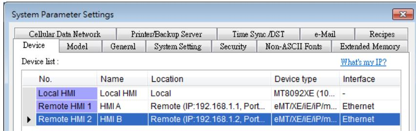
3. Create a Set Bit Object, select “HMI A” in [PLC name] to control the address of the remote HMI A. Same for the HMI B.
