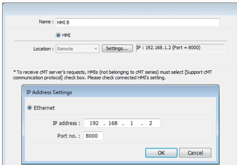
3. In the project of HMI B, go to [System Parameter Settings] » [Device list], click [New PLC], set [Name] to “PLC on HMI B”. Set correct parameters.
