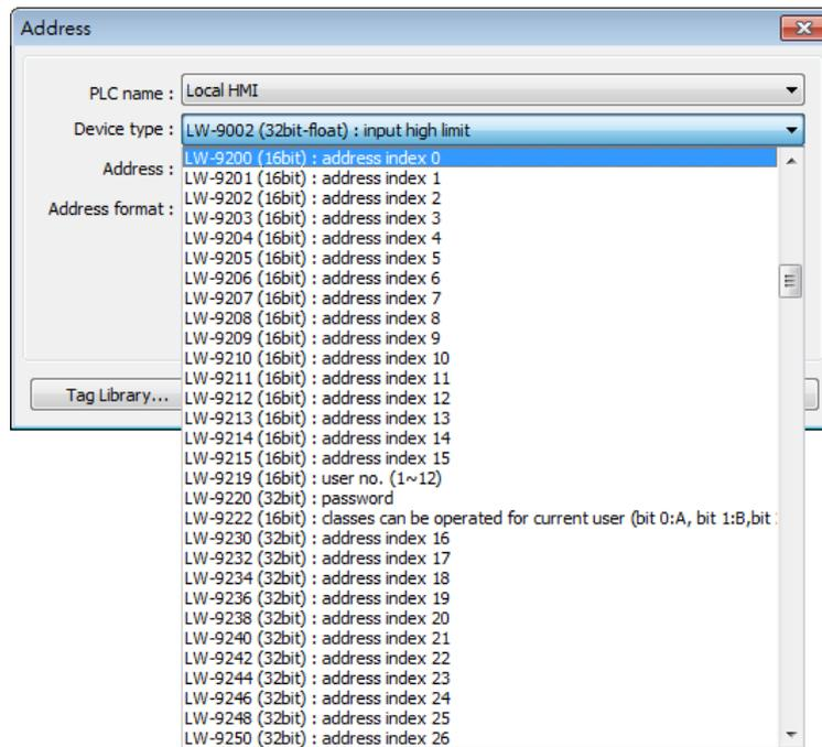
The corresponding address of 16-bit Index Register 0 to 15: LW-9200 (16bit) to LW-9215 (16bit)
