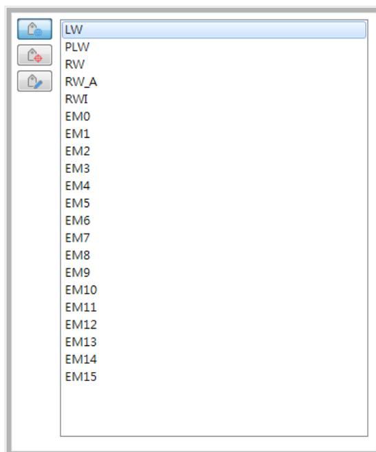
Data in the extended memory is saved as a file into [SD card] or [USB disk]. By default, the files in [EM0] to [EM15] are with the file names “em0.emi” to “em15.emi” respectively, although users are free to change the file names. To open these files and edit the data in the extended memory, RecipeEditor.exe may be used.
