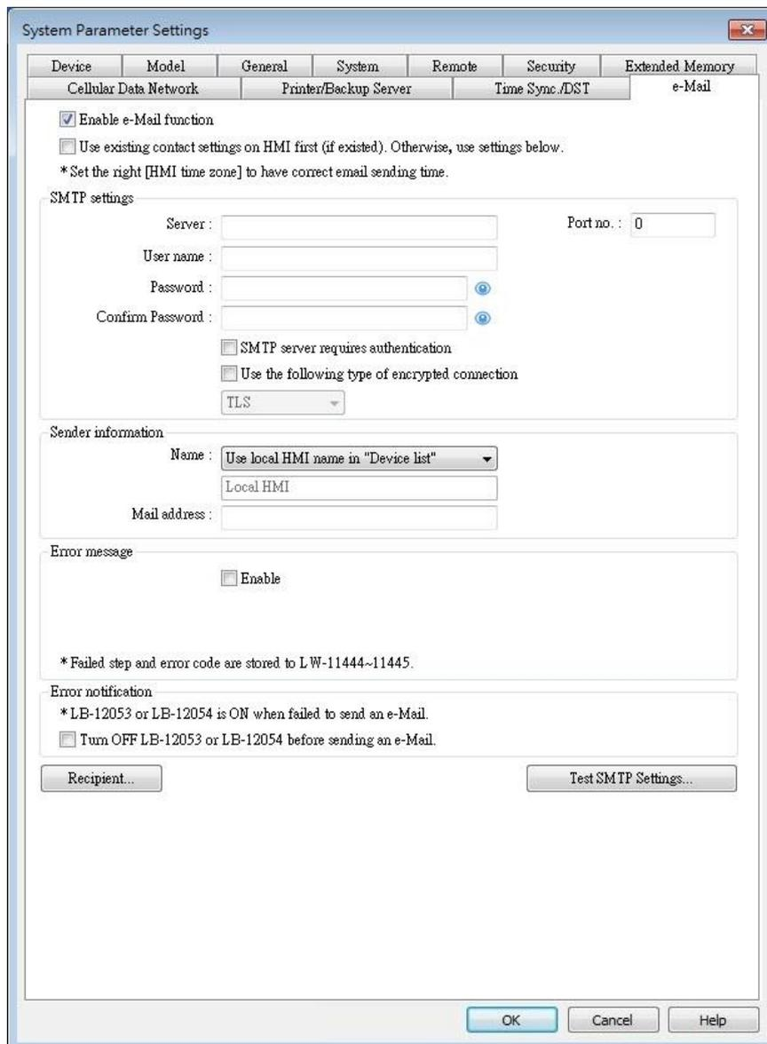
The screenshot shows the 'System Parameter Settings' dialog box with the 'e-Mail' tab selected. The dialog has a tabbed interface with tabs for Device, Model, General, System, Remote, Security, and Extended Memory. The 'e-Mail' tab is active, showing the following settings:
