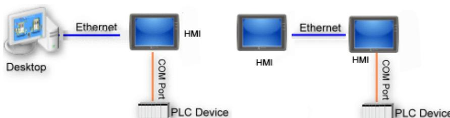
“Remote Device” is a device being connected to a remote HMI. To control a remote device, add this type of device first. Please click [System Parameters] » [New] to open [Device Properties] dialog box. For example, use MODBUS RTU as the Remote Device:
