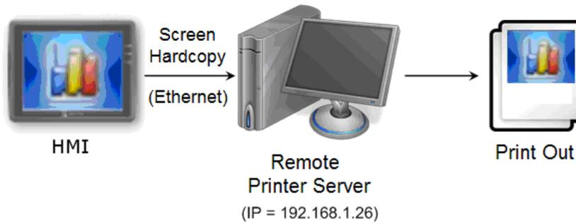
Users can make screen hardcopies with a Function Key object. The hardcopies will be transferred to the Remote Printer Server via Ethernet and then printed out.
