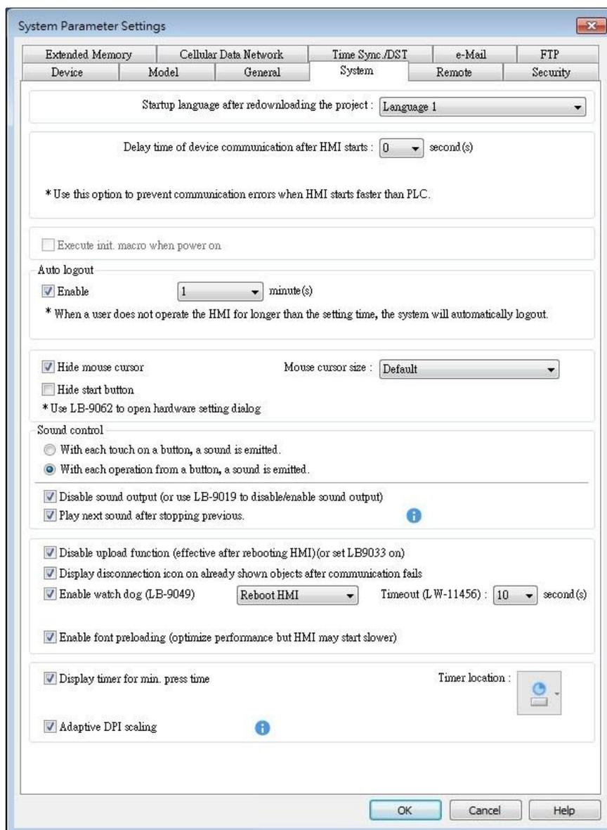
Some features are duplicated from system registers, such as, [Hide system setting bar (LB-9020)], [Hide mouse cursor (LB-9018)], [Disable buzzer (LB-9019)], and [Disable upload function (LB-9033)]. Users can also set these features via system tag.
