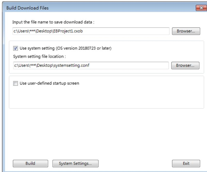
5. Click [Build] to generate a compiled file and a system setting file with the same filename (EBProject1.cxob & EBProject1.conf). Save these files in the same directory in an external device.
