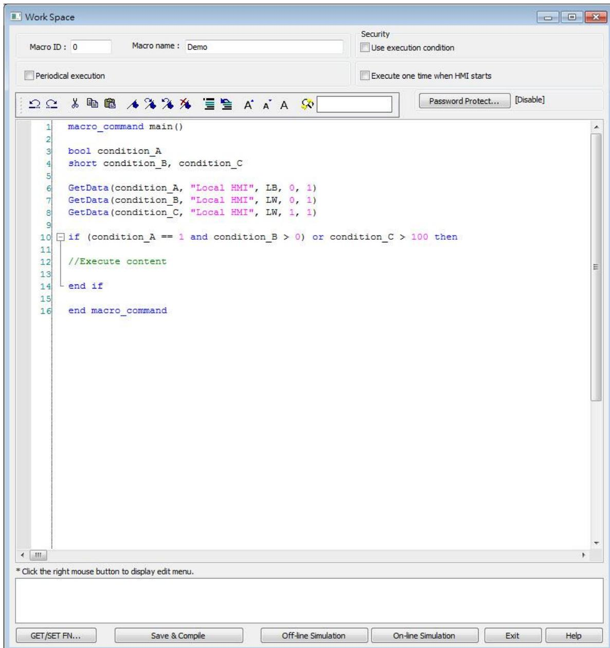
1. Create a Condition object, add condition\_A, condition\_B, condition\_C and then customize a logical expression “( \${1} AND \${2} ) OR \${3} ” as shown below.
