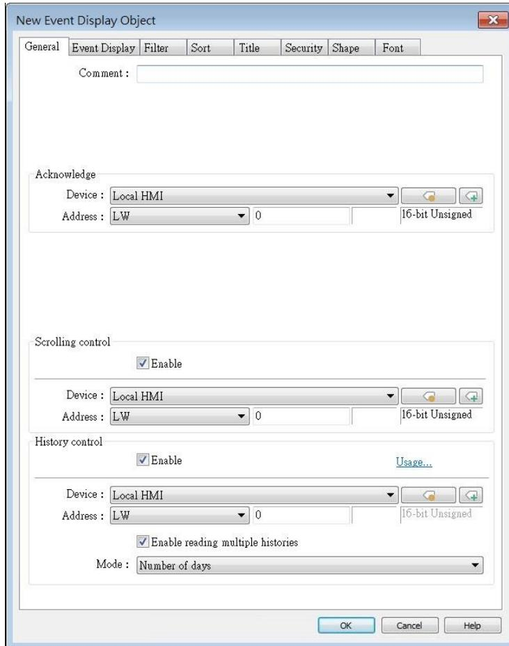
For cMT / cMT X models, only events with “save to history” option selected in the Event (Alarm) Log settings can be displayed in the Event Display object. The events that are not set to be saved in the history can be displayed using the Alarm Bar or Alarm Display object.
