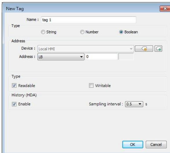
Add a new tag for the client to monitor or control. The name must be specified, and the address can be Readable or Writeable.
