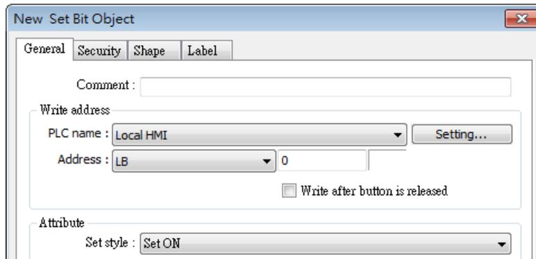
5. Add Set Bit objects on the [Enter] and [ESC] Function Key objects respectively. Set address to [LB-0] and [Set style] to [Set OFF]. In this way when pressing either [Enter] or [ESC] key will close the keyboard window.
