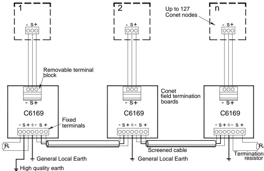
Connections to the C6169 Termination Boards, showing position of the termination resistors. Note Screen is only ever earthed at one point on the Network.
