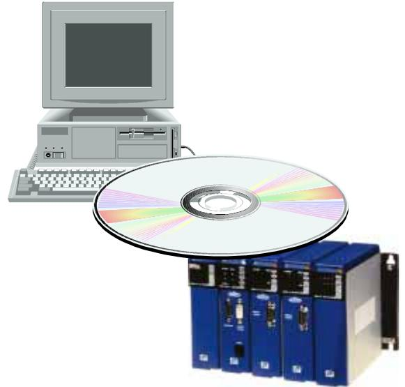
The Omniflex ISaGraf Application Workbench is development software that runs under Microsoft Windows for developing control application programs using the IEC61131-3 standard programming languages.
