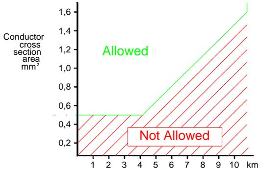
Fig 6: Conet Cable sizing Chart
