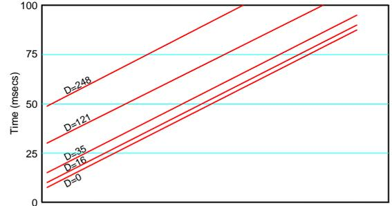
Fig 2: Typical Data Transmission times for a given number of nodes
