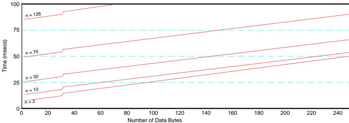
Fig 4: Typical data transmission times for a given number of data bytes transmitted per node per token revolution
