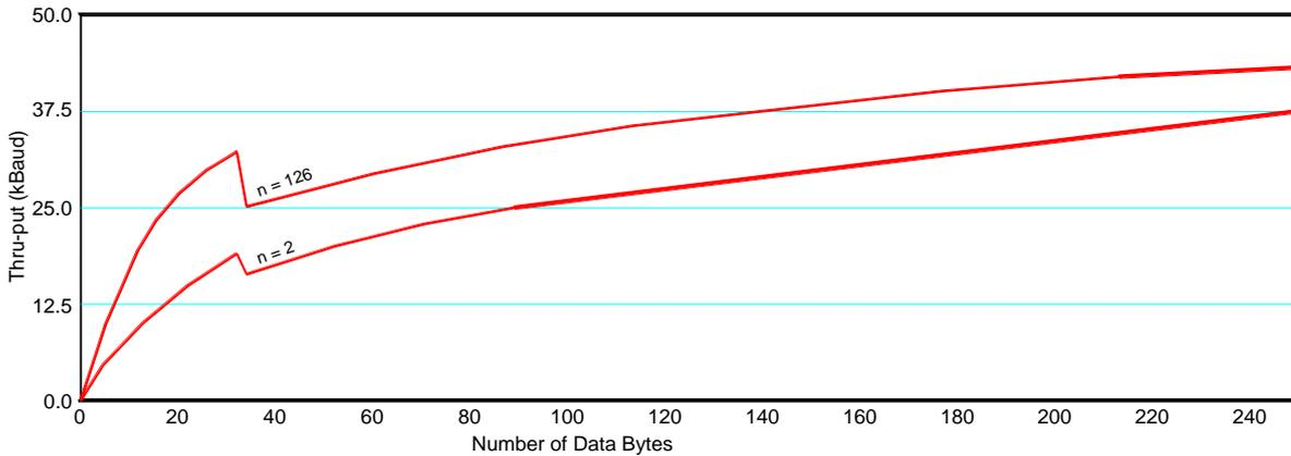
Fig 3: Network thru-put for a given number of data bytes transmitted per node
