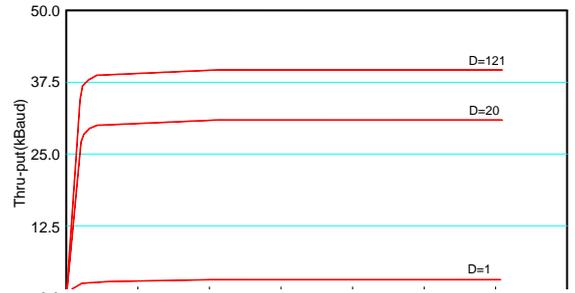
Fig 1: Network thru-put for a given number of nodes
