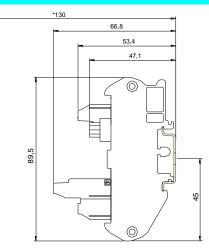
\* NOTE: Allow a total of 130mm from the backplate to accomodate the DB37 connector and cable.
