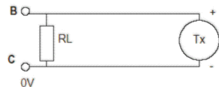
Four-wire transmitter connection
