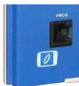
Figure 11.2: Location of Programming Port
