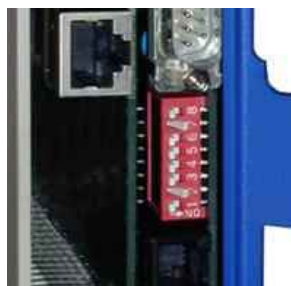
Figure 11.1: Serial Port Address Switch
