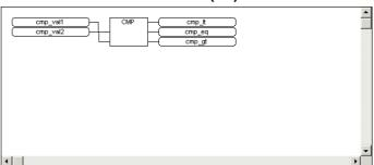
Function Block Diagram (FBD) is a graphical language that allows the user to build complex procedures by taking existing function blocks from the library, and wiring them together on screen.
