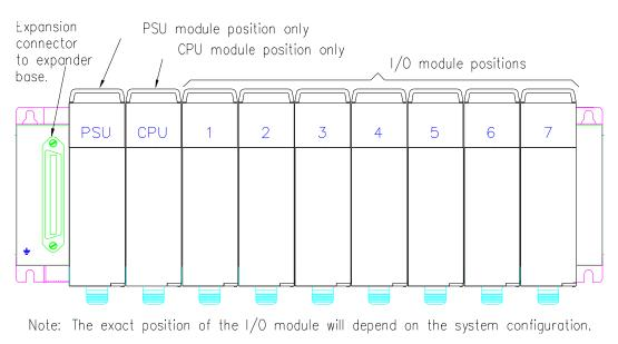
Figure 2.1: Layout of the 7I/O Master Base
