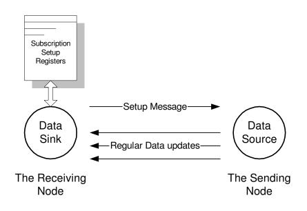
The node acting as a data "source" (the sending node) requires no user configuration to participate in a subscription contract with another node. The node acting as data "sink" (the receiving node) is configured by the user for the required data. The "sink" node then automatically manages the subscription including sending the requests to the data source, and managing errors in the process.
