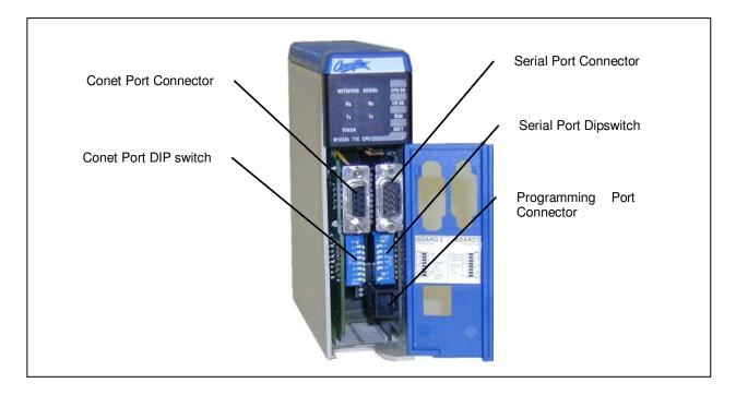
Figure 3.1: View of the M1241B T2C CPU
