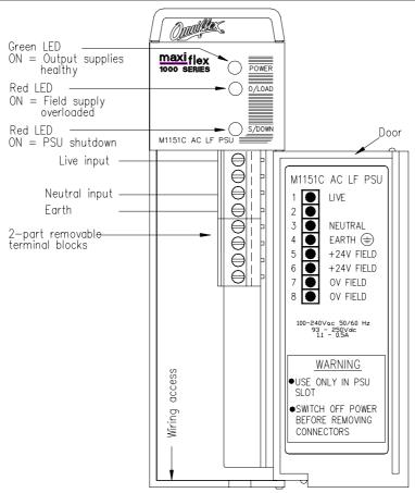
Note: The LEDs can only be seen when illuminated,
