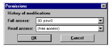
Both permissions can be set either to "free access", or to a protection level defined by a password. Full access permission cannot be attached to a level with less priority than the one selected for read access.
