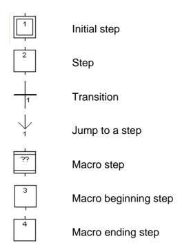
The SFC programming is usually separated into two different levels: The **Level 1** shows the graphic chart, reference numbers of the steps and the transitions, and comments attached to the steps and the transitions. The **Level 2** is the **ST** or **IL** programming of the actions within the steps, or the conditions attached to the transitions. Actions or conditions may refer to sub-programs written in other languages (FBD, LD, ST or IL). Below is an example of level 1 and level 2 programming:
