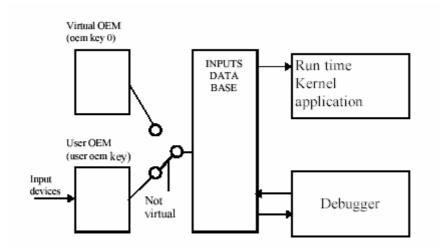
Setting the virtual attribute follows the same rules for an input board or an output board. For output boards, the ISaGRAF kernel updates the output database. This database and the associated output devices are, however, disconnected. A virtual I/O driver replaces the real one.
