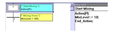
The level 2 programming of a step is entered in a text editor. It can include action blocks programmed in ST or IL. The level 2 programming of a transition can be entered either in IL or ST text languages, or with Quick LD editor.
