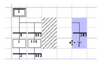
The destination area for moved elements must be empty. No insertion is possible while moving SFC symbols.
