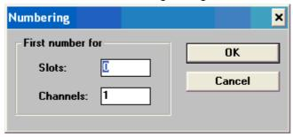
As default, slot numbering starts at index "0", and channel numbering starts at index "1"
