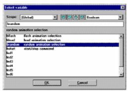
The "Scope" selection box is used to select between global and local variables. The selection box on the right allows the selection of the data type. Small icons beside the type selection box are buttons that can be used as shortcuts to select most current data types:
