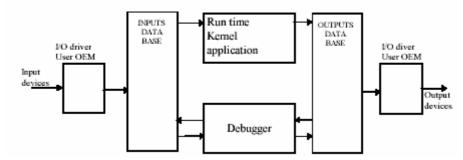
When an input variable is locked, the various accesses to the database are not changed, but the input device is disconnected. Input values can be set with the debugger and processed by the ISaGRAF kernel:
