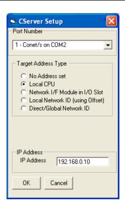
An IP Address is only required if communicating using Conet/e over Ethernet.
