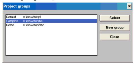
Select a group in the list and press "Select" to activate it in the project management list. You can also double click on its name to select it. Use the "New group" command to create a new group. This command can be used either to assign a group name to an existing directory, or to create a new group with a new directory.
