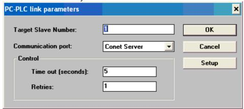
5. Select "Setup" and then choose the desired Conet Port for communicating with the P3 CPU. Programming can be performed over Conet/s (through a serial port on the computer), Conet/c(through a Conet/c Interface Card if installed on the computer and Conet/e(through an Ethernet port if installed on the computer).
