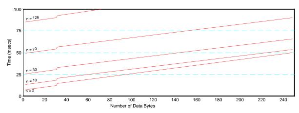
Fig 4 : Typical data transmission times for a given number of data bytes transmitted per node per token revolution
