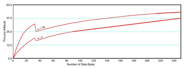
Fig 3: Network thru-put for a given number of data bytes transmitted per node
