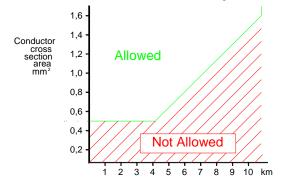
Fig 6: Conet Cable sizing Chart
