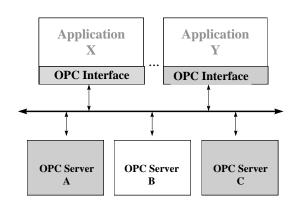
Multiple Applications from different software vendors can now communicate simultaneously with multiple hardware devices using an OPC Interface between the software applications and the OPC Servers.
