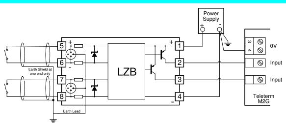
Example 1: Interfacing field contact inputs to a Teleterm M2 Series RTU
