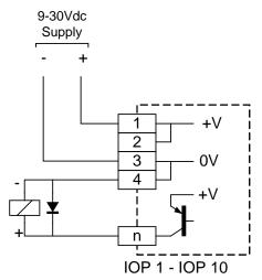
Figure 2.3 - Digital Output Connections
