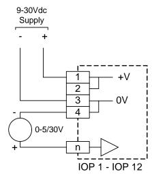
Figure 2.4 - Analogue Input Connections
