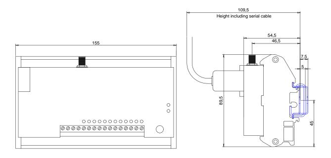
Figure 2.1: Mechanical Mounting Dimensions for the Teleterm M2
