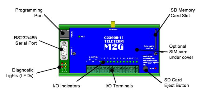
Figure 1.1: Front View of the Teleterm M2G with internal GSM modem
