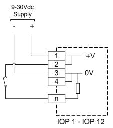
Figure 2.2 - Digital Input Connections
