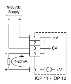
Figure 2.5 - Analogue Output Connections
