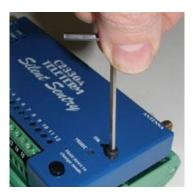
Insert the SIM card into the SIM card holder you will see in the centre of the unit. Take special care that the SIM card is correctly seated in the connector, and that the SIM card holder is properly closed. Press firmly down and slide forward to close securely.
