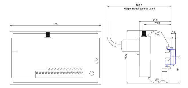
Figure 2.1: Mechanical Mounting Dimensions for the Silent Sentry
