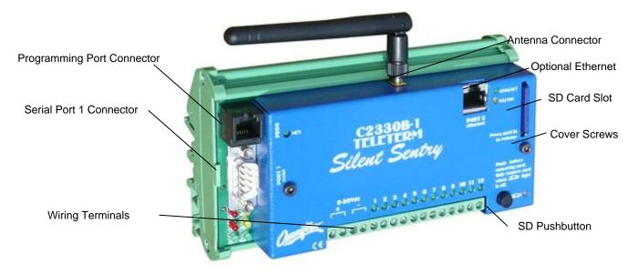
Figure 1.1: Front View of the Teleterm Silent Sentry with Ethernet port
