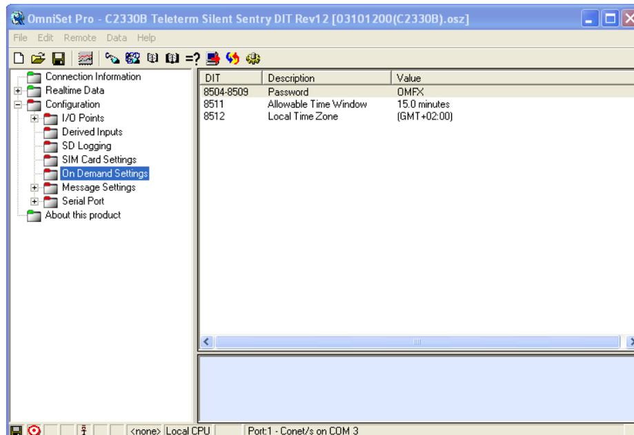
The default factory password is OMFX, but this should be changed immediately. This password needs to match the password in the On-Demand message sent to the RTU. On-Demand messages sent to this unit must contain this password for the messages to be accepted. This password is NOT case sensitive.(i.e. ABC = abc). Up to 12 characters can be used.
