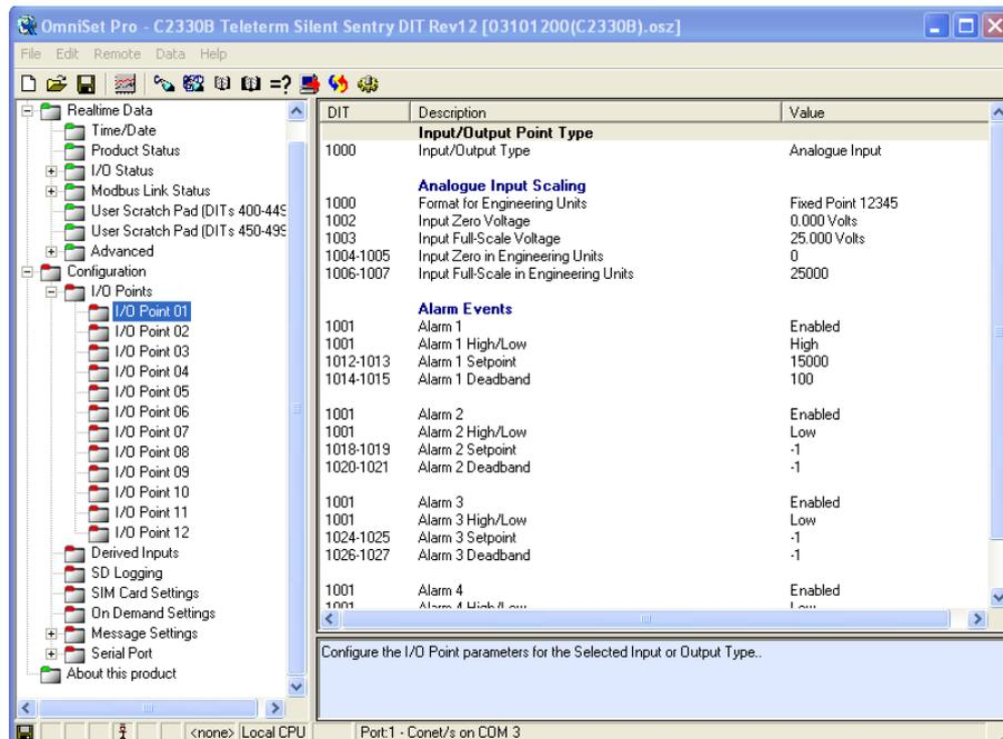
1. Set the scaling to scale the Input Voltage to engineering units.
