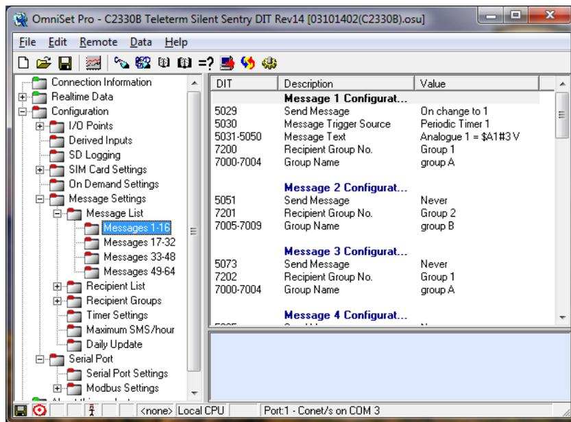
In the above example, the value of Analogue Voltage 1 (formatted to 3 decimal places) is embedded in the message by using “\$A1#3” in the message text.
