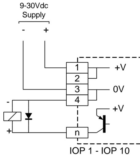
*Figure 2.3 - Digital Output Connections*
