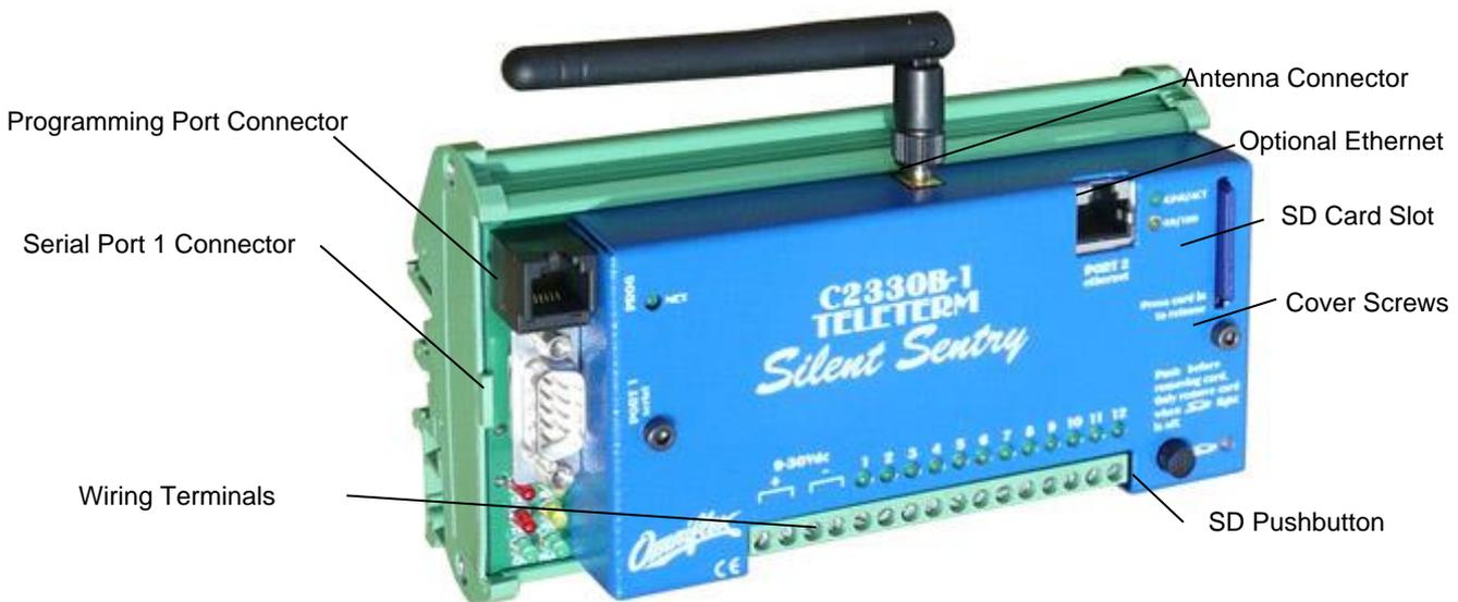
*Figure 1.1: Front View of the Teleterm Silent Sentry with Ethernet port*
