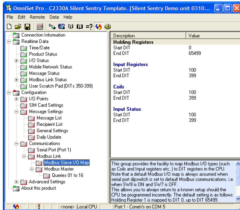
The most efficient data type to use is Holding Register Read (Modbus Function 3) and Holding Register Write (Modbus Function 16).
