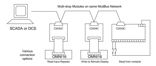
Typical System Diagram showing various connection options.
