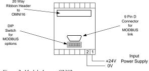
Figure 2: Module Layout C2302
