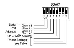
Figure 4-3 Serial Port Settings on SW2
