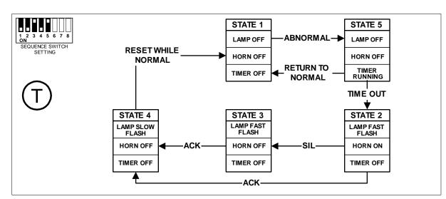
Sequence 11 - Momentary (Fleeting) Alarm; Manual Reset; for Motor Alarms; with Time Delay on Inputs
