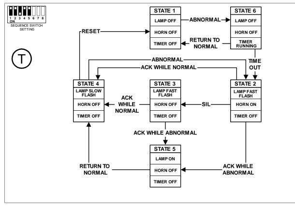
Sequence 4 - Momentary (Fleeting) Alarm, Manual Reset, with Ringback, Timer Delay on inputs.
