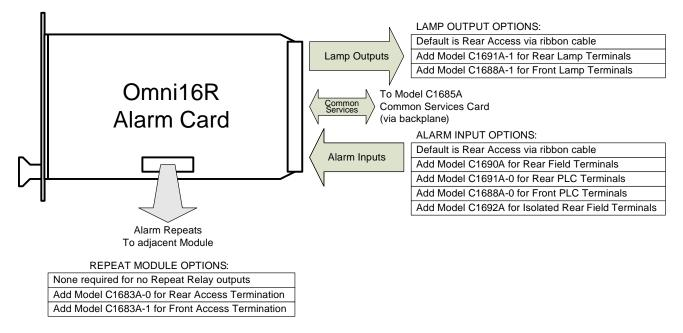
Figure 1-5 – Omni16R Side View showing available connections
