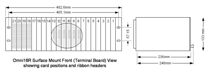
Figure 1-4 – Surface Mount Omni16R Front View showing card positions
