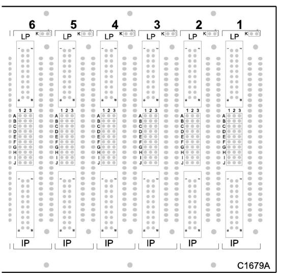
Figure 1-6 – Motherboard View showing link fields.
