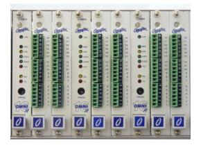
Figure 1-2 The Omni16R Cards with front termination
