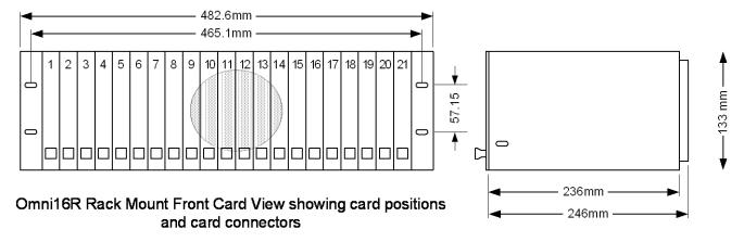
Figure 1-4 – Panel Mount Omni16R Front View showing card positions
