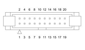
Figure 3-8 Ribbon Header Pin Layout
