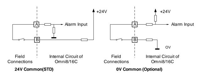
Figure 3-3 Input Connection Diagram using individually wired Potential Free Contacts
