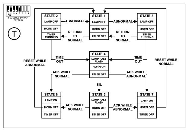
Sequence 13 - Pulse Monitoring Alarm, Manual Reset
