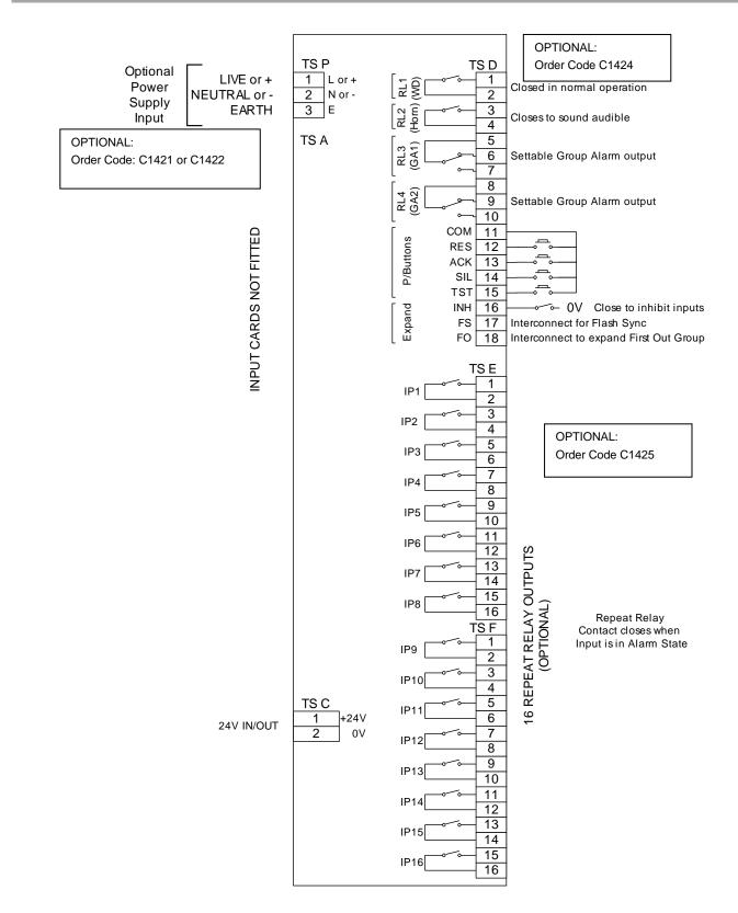
**NOTE:** Facilities provided on Terminal Strips TS-P, TS-D and TS-F require options to be ordered in addition to the standard serial display unit.
