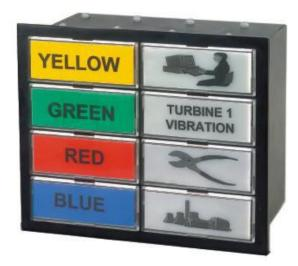
for N.O. or N.C. operation. Inputs are wired to plug-in terminals at the rear of the annunciator. The alarm sequence for the 8 inputs is also configured by DIP switch with a choice of 27 standard sequences. Four output relays can be configured as group alarm, horn output and watchdog with a change over contact at the terminals. The group alarm can be set to one of four functions, Follows input, follows alarm, Multiple reflash, Ringback horn.
