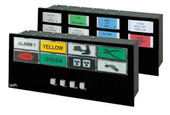
or 90-150 Vac/dc are also available. The alarm sequence for the 8 alarm points is configured by DIP switch with a choice of 27 standard sequences. Four relay contact outputs provide group alarm, horn and watchdog outputs. The group alarm can be set to one of four functions: follows input, follows alarm, Multiplereflash or Ring-back horn.
