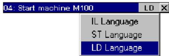
A single line edit box appears at the top of the level 2 window. It is used to enter a short description text. This text will be displayed as an IEC comment in the drawing of FC symbols. It is very useful as it is used by other commands such as "Go To..." and also in the FC printout to document FC actions and tests.
