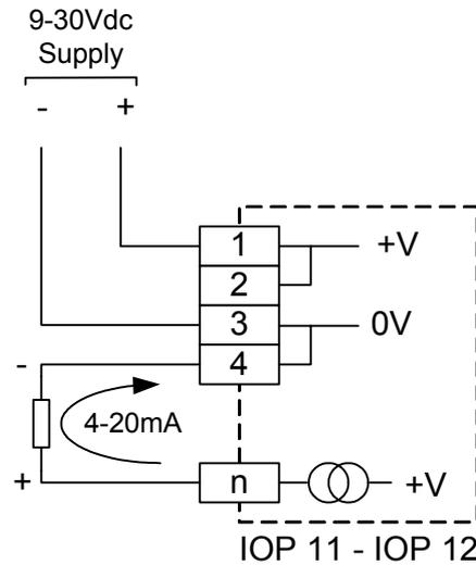
*Figure 2.5 - Analogue Output Connections*
