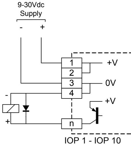
Figure 2.3 - Digital Output Connections
