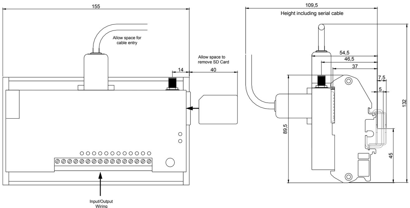
**Figure 2.1: Mechanical Mounting Dimensions for the Teleterm M2**
