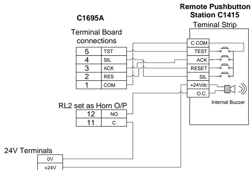
**Figure 3-6 Connecting C1415 Remote Pushbutton Station to Omni16R units.**
