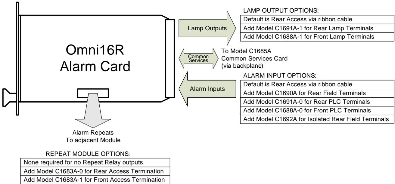
*Figure 1-5 – Omni16R Side View showing available connections*
