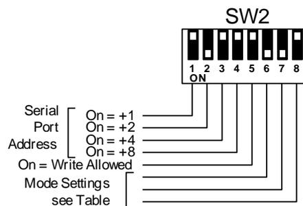
*Figure 4-3 Serial Port Settings on SW2*
