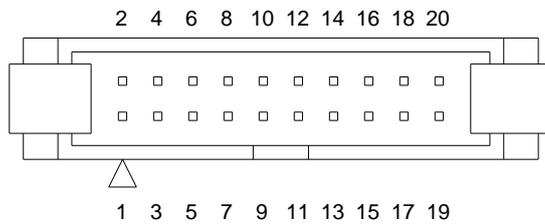
**Figure 3-8 Ribbon Header Pin Layout**
