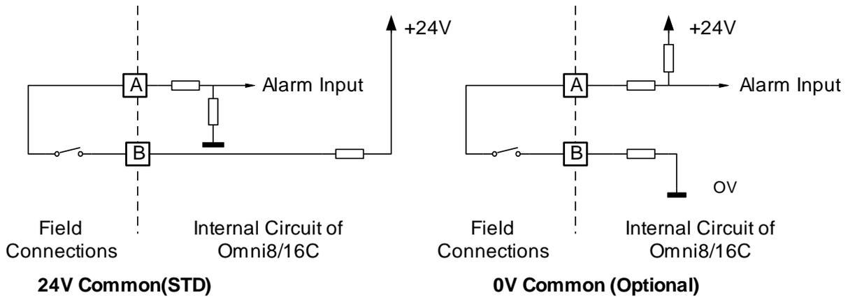
**Figure 3-3 Input Connection Diagram using individually wired Potential Free Contacts**
