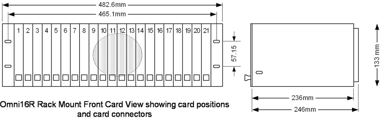
*Figure 1-4 – Panel Mount Omni16R Front View showing card positions*
