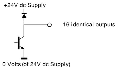
**Figure 3-7 Open Collector Transistor Output Arrangement**
