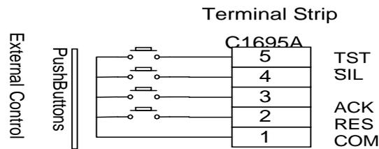
**Figure 3-5 External Pushbuttons controlling a single Omni16R**
