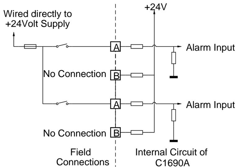
**Figure 3-4 Input Connection Diagram using Common Return Wire**
