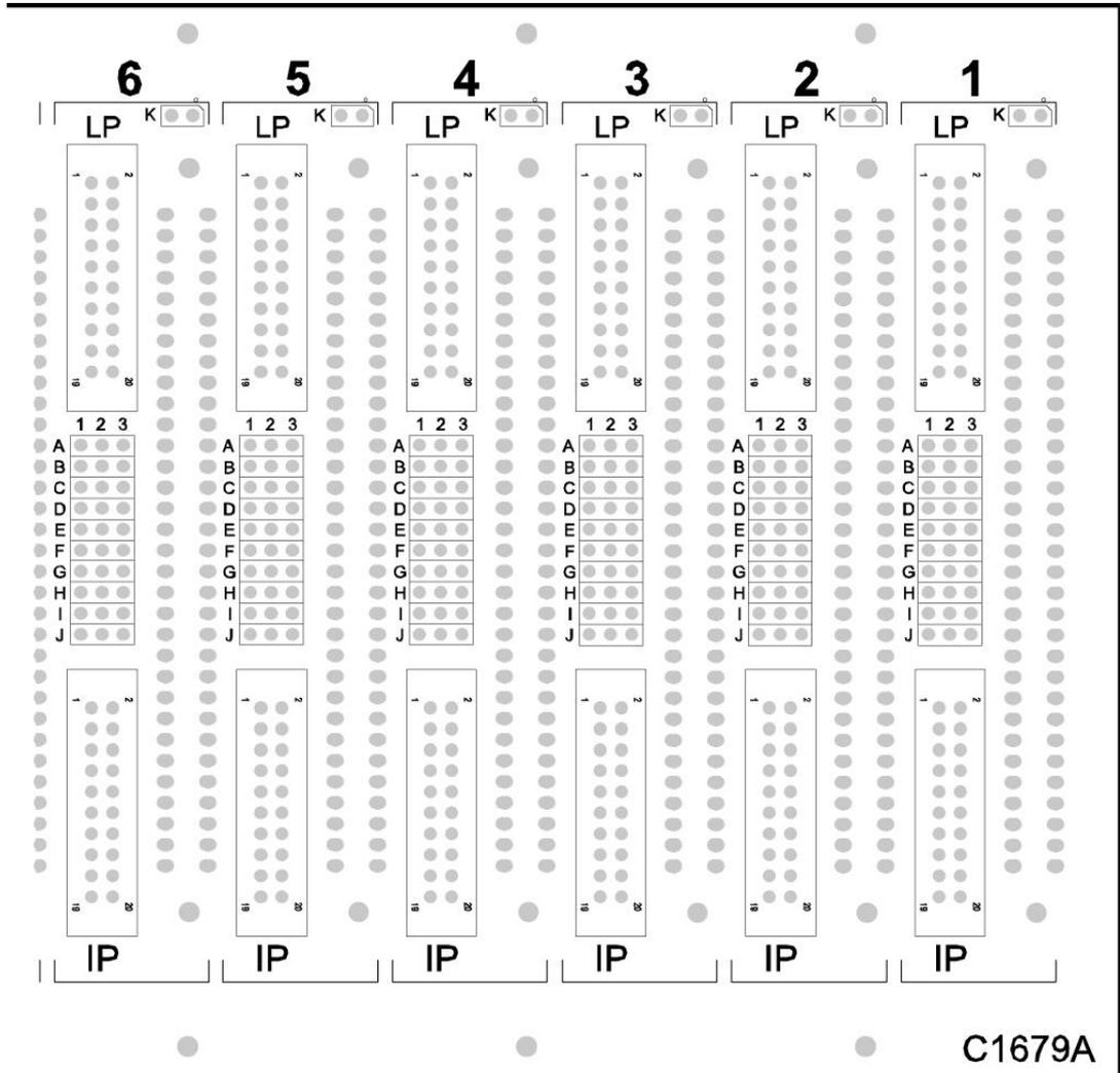
Figure 1-6 – Motherboard View showing link fields.
