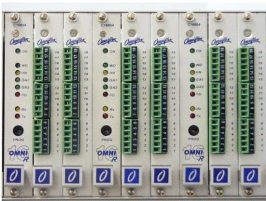
**Figure 1-2 The Omni16R Cards with front termination**
