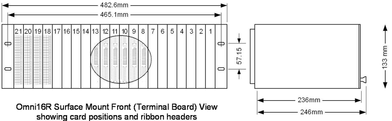
*Figure 1-4 – Surface Mount Omni16R Front View showing card positions*
