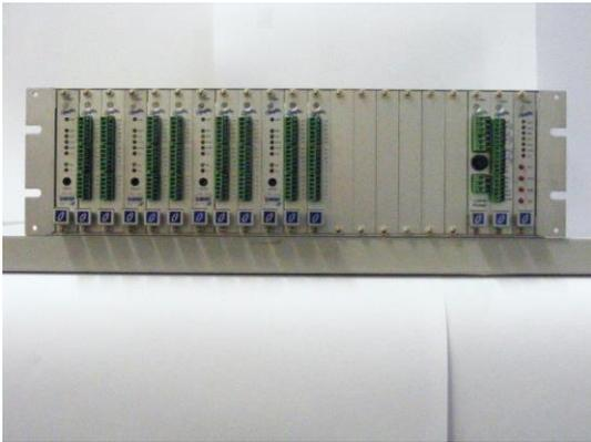
**Figure 1-1 The Omni16R 19" Rack Mount Alarm Annunciator system.**
