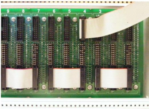
**Figure 1-3 The Omni16R 19" Rack Mount rear link area.**
