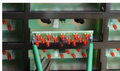
2. Pull the board out by its edges
