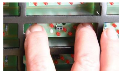
3. Press the LED Board on to the retaining clip
