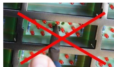
3. Do NOT attempt to pull the LED board out by its central connector.
