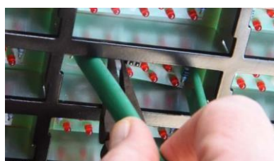
1. Grab the LED board by its edges while squeezing the barb on the retaining clip
