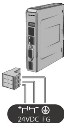
**Note:** Connect positive DC line to the ‘+’ terminal and the DC ground to the ‘-’ terminal.
