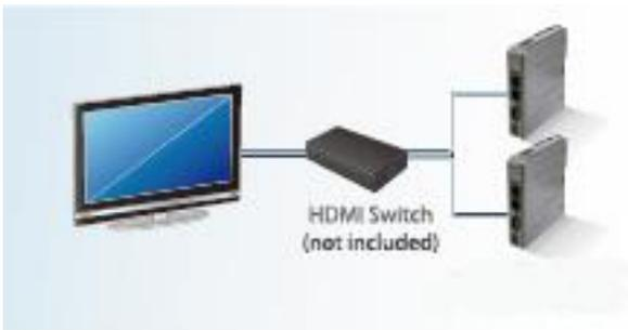
**Note:** If not connecting a repeater, the maximum length of HDMI cable allowed is 15m. To reach a longer distance, please use CAT6 cable or a repeater. HDMI converter is used to detect the monitor and correctly output.
