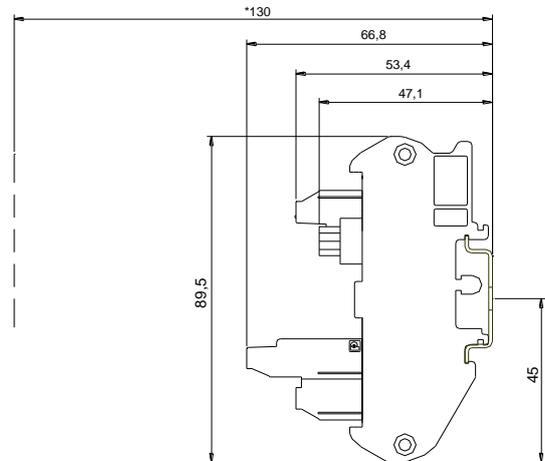
\* NOTE: Allow a total of 130mm from the backplate to accommodate the DB37 connector and cable.
