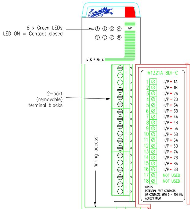
Note: The LEDs can only be seen when illuminated, as they are located behind the LED cover.
