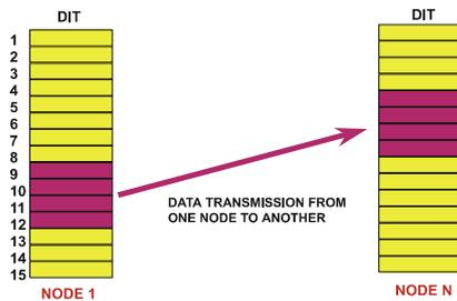
In all these cases, the traditional method is for a controlling master node to poll the slave nodes regularly for data in case something has changed. This crude method is an inefficient use of the limited network bandwidth, and is inherently slow in typical update times. The MAXIFLEX A3 CPU provides a superior mechanism to accomplish this commonly used function, through its Subscription Service.
