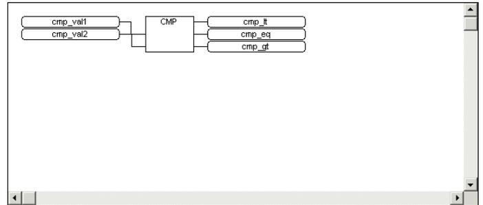
Function Block Diagram (FBD) is a graphical language that allows the user to build complex procedures by taking existing function blocks from the library, and wiring them together on screen.
