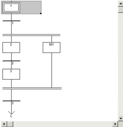
Sequential Function Chart (SFC), the core language of the IEC 61131-3 standard, divides the process cycle into a number of well-defined steps, separated by transitions. The other languages are used to describe the actions performed within the steps and the logical conditions for the transitions. Parallel processes can easily be described using SFC
