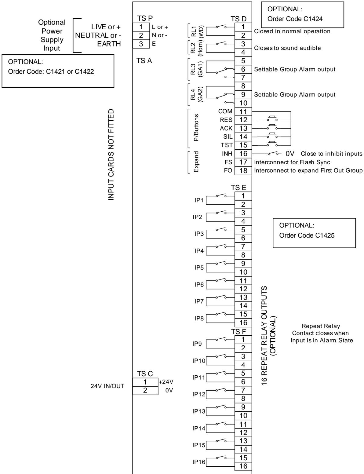
**NOTE:** Facilities provided on Terminal Strips TS-P, TS-D and TS-F require options to be ordered in addition to the standard serial display unit.
