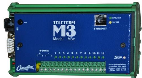
Basic Teleterm M3e RTU with 10/100 Ethernet Port (Model C2360B-0)
