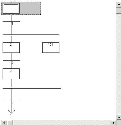
Sequential Function Chart (SFC), the core language of the IEC 61131-3 standard, divides the process cycle into
