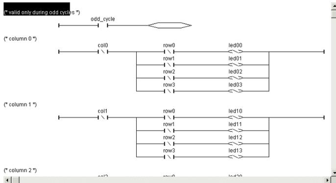
The Ladder Diagram (LD) is one of the most familiar methods of representing logical equations and simple actions, particularly in the United States. Contacts represent input arguments and coils represent output results. The Workbench's Quick LD editor provides the best compromise between high-level graphic capabilities and easy-to-use keyboard driven programming. LD and FBD programming can be mixed in the same chart.
